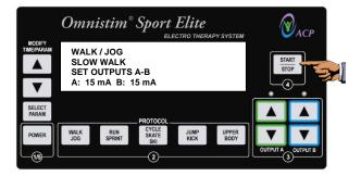
7). When the desired output the timer will start to begin timed treatment mode. At this time, the timer display on the right side of the screen will display the selected treatment time, and will continuously display time remaining, in minutes, during treatment.
