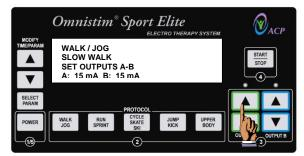
**6).** Adjust the output by pressing the OUTPUT A and OUTPUT B UP or DOWN buttons (3), to deliver appropriate output based on patient sensation.
