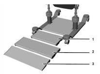
All tread extensions do not need to be used, however the connection part must be used to use the additional tread extensions.
