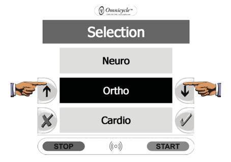
Pressing the UP or DOWN arrows will scroll the screen thru the available main programs: Neuro, Ortho, Cardio Soccer, Porcupine, Traffic Jam, and System. To select the desired program, press the CHECK MARK ('1) button when that program appears in the screen center, and is identified by the black color of the program name box.
