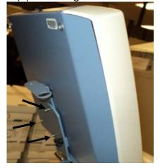
13. Plug in the terminal. Plug in the cycle power cord from the original cycle.
