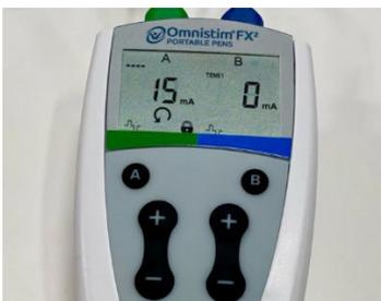
**NOTE:** To readjust stimulation intensity, remove the lock by pressing (-) Button and then (+) Button to preferred level.
